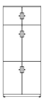
342mm (13.5") high doors = 318mm (12.6") 380mm (15") high doors = 354mm (13.9") 684mm (26.9") high doors = 661mm (26") 760mm (29.9") high doors = 740mm (29.1")
