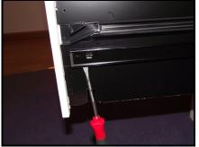
Insert a flat head screwdriver underneath the front of the runner as shown. You could also insert from the top whichever you find easier.
