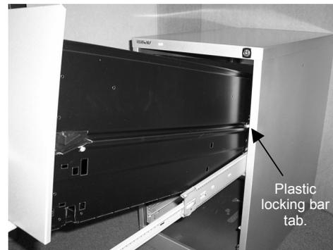
Slide the drawer backwards into the cabinet, raising the front to locate the right side edge of the drawer underneath the plastic locking bar tag.
