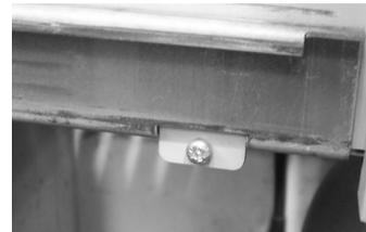
Lower the front of the drawer, lining up the tabs with the slots in the suspension slide inner members. Fit screw and tighten.
